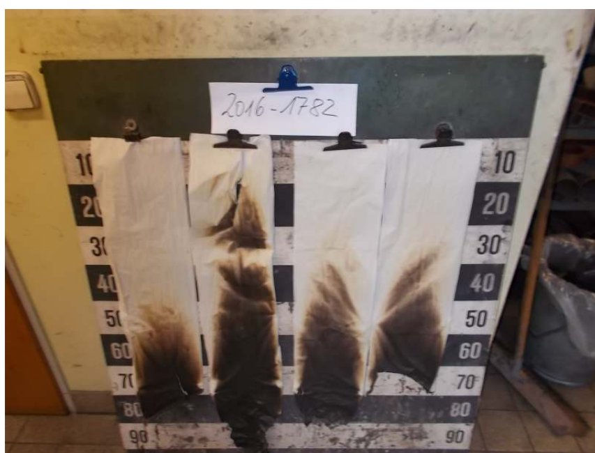
appearance of the sample C after the Brandschacht test
