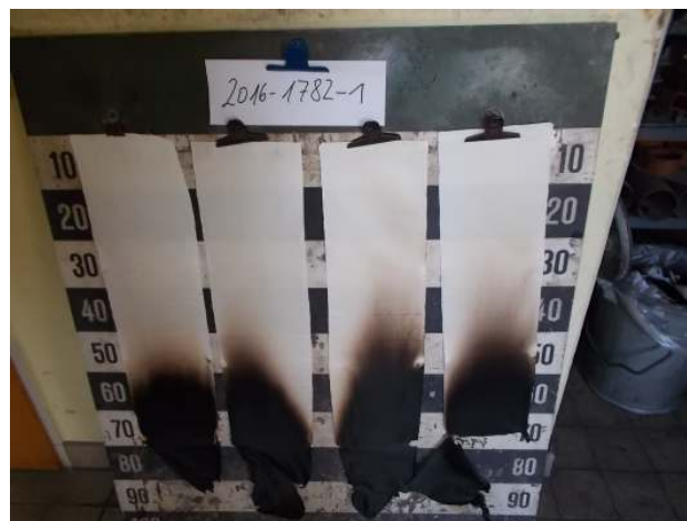
appearance of the sample B after the Brandschacht test
