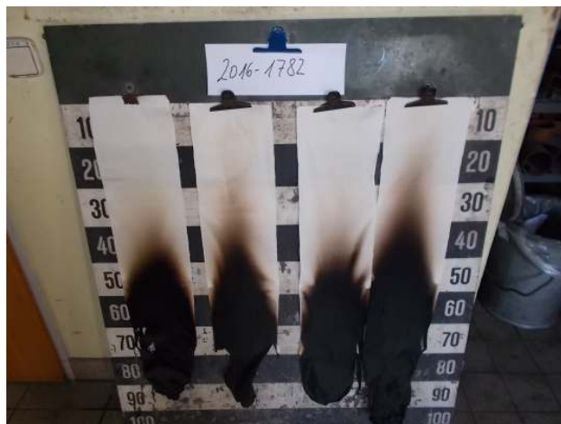
appearance of the sample A after the Brandschacht test
